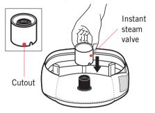
The Sleeve concentrates a small amount of water around the Exposed Heating Element, quickly bringing it to boiling temperature to produce steam, rather than heating all of the water in the reservoir.
